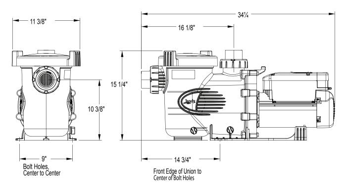
**NOTE** When installing a pump, leave a minimum of two feet (2 ft) of clearance above the pump for removal of the strainer basket.
