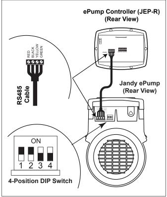
Figure 2. Wiring ePump Controller (JEP-R) to ePump
