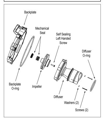
Figure 13. Backplate, Impeller, Diffuser, Mechanical Seal Exploded View
