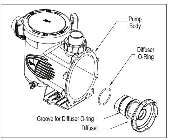
Figure 12. Pump Body and Diffuser Exploded View
