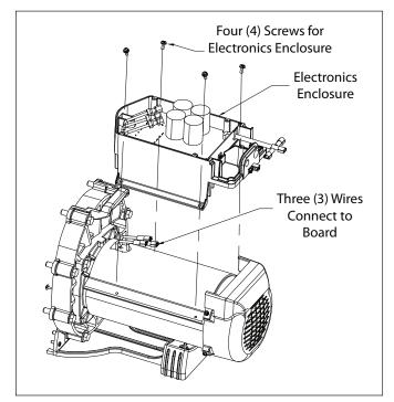
Figure 15. Remove Variable Speed Drive Electronics Enclosure
