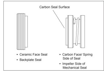
Figure 11. Mechanical Seal
