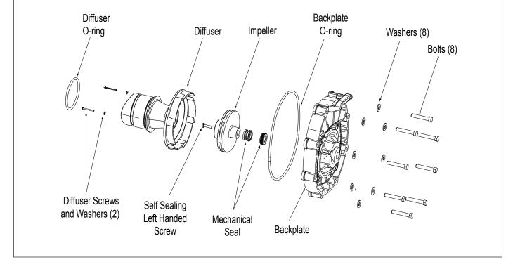
Figure 10. Diffuser and Impeller Exploded View
