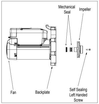
Figure 9. Remove the Impeller
