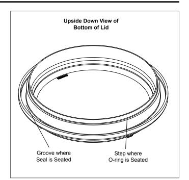
Figure 6. Placement of Blue Pressure Test O-ring
