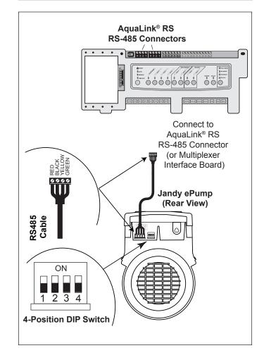
Figure 3. Wiring AquaLink® RS Controller or AquaLink<sup>®</sup> PDA to ePump
