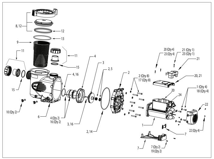
Figure 17. ePump Exploded View
