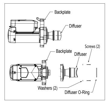
Figure 8. Remove the Diffuser
