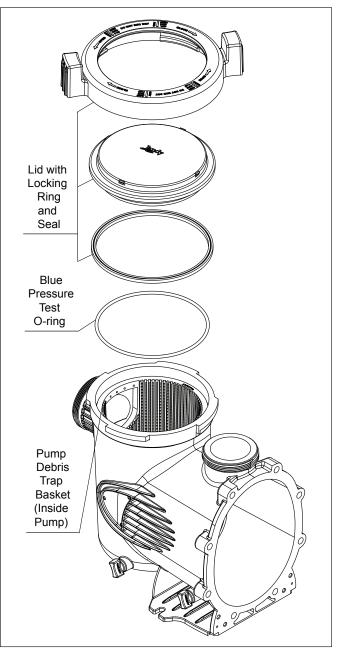
Figure 5. Exploded View of Pump
