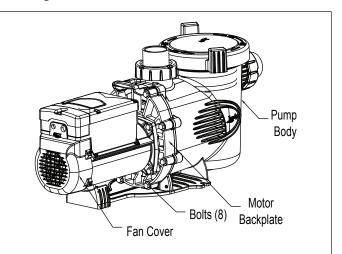
Figure 7. Remove the Pump Housing
