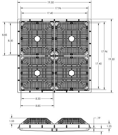
Part No. Description 819-1031 #8 x 1 Stainless Steel Screw 642-479X V 9" x 9" Grate **642-474X** 18" x 18" Grate Frame
