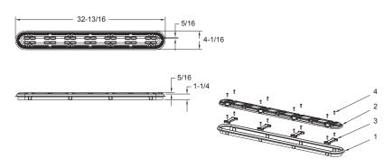
1. 32" channel drain, no sump, frame
