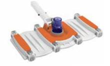
Triangular vacuum head with EZ-clip. Swiveling platform avoids twisting of hose and orients vacuum head along walls. Vortex shaped underside plate and extra underside brushes in 2 densities increase vacuum efficiency. Fits 1-1/4" & 1-1/2" vacuum hose.
