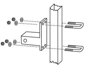
YOUR TRUCK MUST HAVE A 2" HITCH TO USE THE INCLUDED RECEIVER. IF YOU HAVE A 2" HITCH, THEN FOLLOW THE MOUNTING DIAGRAM ABOVE. ADJUST THE HEIGHT OF YOUR HAMMERHEAD MOUNT AS IS APPROPRIATE.
