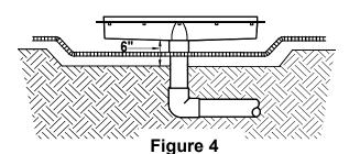
When Using 2 1/2" Suction Add 6" More to Determine the Riser Cut-Off Point (Pool Depth Plus 9" From the String)
