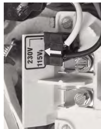
Figure 5B Voltage Change Plug Set for 115 Volts
