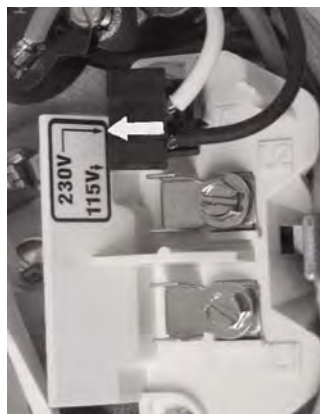
Figure 5A -Voltage Change Plug Set for 230 Volts
