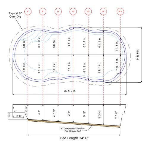
The first step is to define the center line of the pool. Once you have worked out where you intend to locate the pool place a steel pin into the ground at the proposed location of the center of the shallow end and at the proposed center of the deep end. Run a string line from the shallow end steel pin to the deep end steel pin. Measure the distance of the string line to ensure that is the correct length of the swimming pool.
