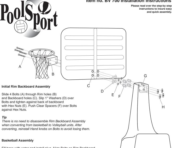
Fill base with water and install plug. Align Bolts on Rim Backboard Assembly with Post Holes (G) and slide through, securing with Hand Knobs (H).
