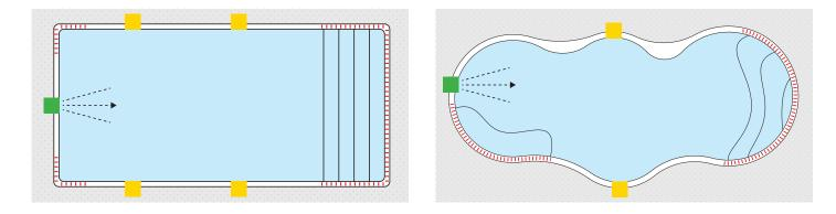
\*Reminder: BADU SwimJet Systems require a clear **unobstructed** area within the swimming pool that is 8 feet wide x 15 feet long x 3 feet deep to work effectively. This "swimming envelope" allows enough length for a swimmer to comfortably drift back and swim against stream.
