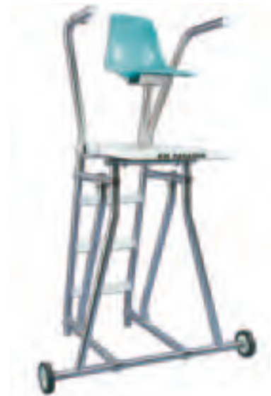
Rover SemiPermanent Designed for those pools where the lifeguard chair must be anchored, yet still be capable of being readily moved. (In Sunbelt states chair might be moved to opposite sides of the pool each day to keep the sun out of the guard's eyes.) The rear legs are set into sockets anchored in the deck, while the front legs with 7" diameter wheels allow for easy relocation. Ladder has 19" steps. Furnished with two pairs of anchor sockets (for two locations), additional sets must be ordered separately. I.D. No. 20303 Spec Sheet LG 20.33
