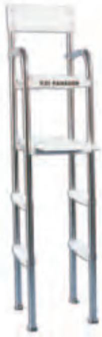
Standard Our original, basic guard chair. The seat, backrest, and non-skid footrest are fabricated of laminated wood coated with fiberglass and polyester resin. The frame is constructed of stainless steel tube and ABS steps. Platform height is 4'4" and seat height is 6'0" above the deck. Furnished with a 19" step and holders for rescue tube and umbrella. Optional anchors and escutcheon plates available. I.D. No. 20601 Spec Sheet LG 20.35
