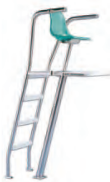
Paraflyte Ladder at Rear Recommended for general use. The rear ladder with flared guard rails provides easy access to the platform. The horizontal rails provide protection and serve as arm rests. Paraflyte (Ultraflyte) Chair I.D. No. 20001 Stainless steel rails are .145" wall Paraflyte (Superflyte) Chair I.D. No. 20002 Stainless steel rails are .065" wall Spec Sheet LG 10.41
