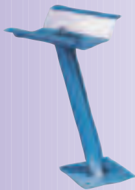
Swivel Chair Seat Support Stainless steel welded assembly ready for installation. Designed to render proper seating angle when mounted to plastic seat. Has 360° swivel capability with bearing surface of low friction non-metallic disc to prevent seizing or binding due to corrosion. Rugged construction. I.D. No. 20702
